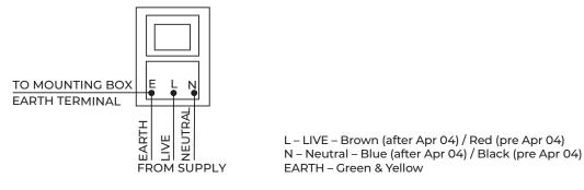
All earth connections must be made and maintained. Use green/yellow sleeving on earth conductors that are not insulated.
