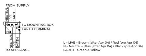
All earth connections must be made and maintained. Use green/yellow sleeving on earth conductors that are not insulated.
